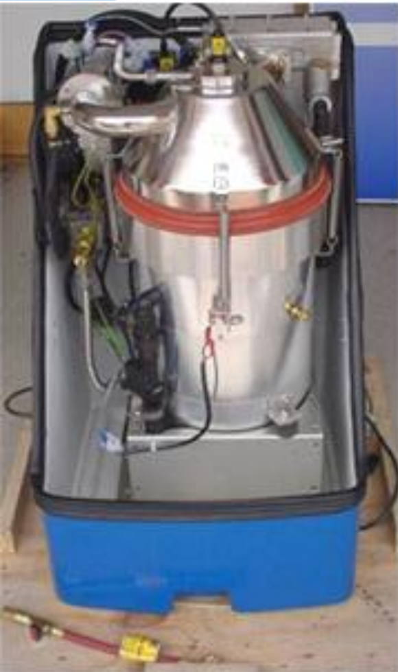
Stirling Engine - the first micro CHP plant tested at CCHT
